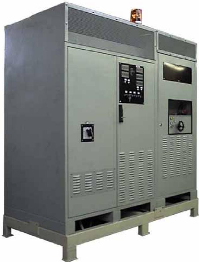
The purpose of the apparatus is to provide, from the mains voltage 400V, the four voltages employed on the European carriage: 3000Vdc, 1500Vdc, 1500Vac and 1000Vac 16,6Hz. These voltages are stabilized and manually settable.
